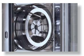
Eloma's high-performance dual humidity generator uses a microsprayer to create just the right amount of steam for perfect humidification. Dual injection onto a rotating sprayer guarantees extremely fast humidity saturation in the entire baking chamber.
